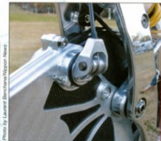
Revised shifter: Earlier Honda gearboxes used an external rotary shift device. The '04 version's cable enters the housing in a cleaner fashion.
